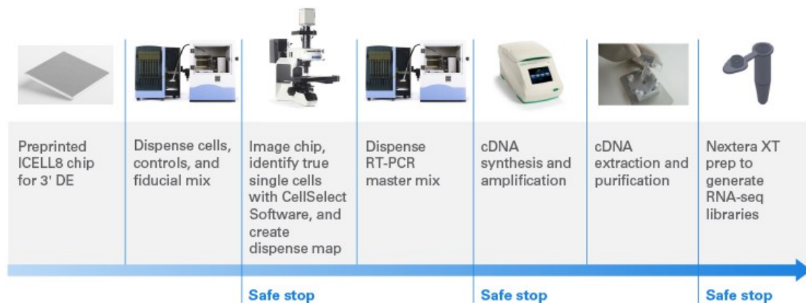
Figure 1. ICELL8 Single-Cell System workflow overview. Cells, controls, and fiducial mix are dispensed onto a 5,184-well chip at an average of one cell per well. CellSelect Software automatically identifies nanowells containing live, single cells and creates a dispense map targeting only these wells, saving time and reagents. Targeted nanowells are then subjected to cDNA synthesis, with a barcode in each well allowing the association of sequencing data with a given cell. cDNA is extracted and purified, RNA-seq libraries are generated via PCR off-chip, and then libraries are subjected to sequencing.
