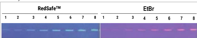
Fig. 3. Gel analysis of serially diluted genomic DNA using RedSafe™ Nucleic Acid Staining Solution (20,000x) and EtBr
