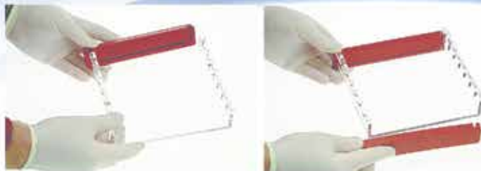
Casting dams allow gels to be rapidly cast
