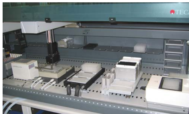
Figure 3: Worktable layout: Sample area, magnetic bead separator, Te-VacS vacuum station, cooled carrier, reagent area, disposable tip area, heating block (from left to right).
