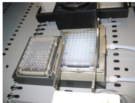
Figure 2: Te-VacS vacuum extraction module for use of M-N NucleoSpin Viral RNA Kit.
